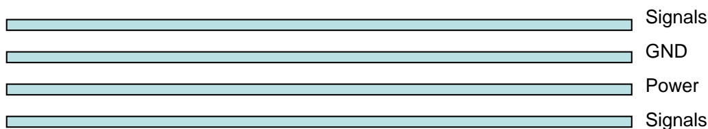
Figure 14: Typical 4-layer PCB construction
