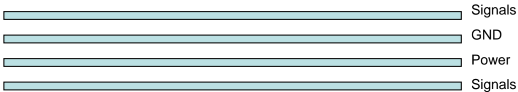
Figure 17: Typical 4-layer PCB construction
