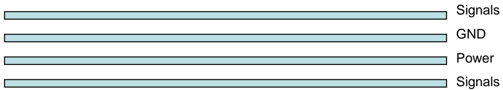
Figure 18: Typical 4-layer PCB construction
