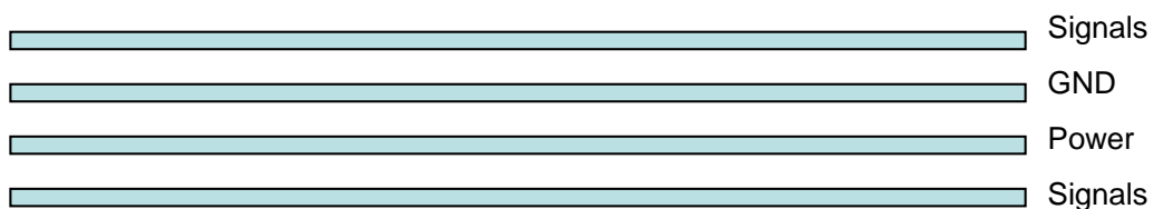
Figure 7: Typical 4-layer PCB construction
