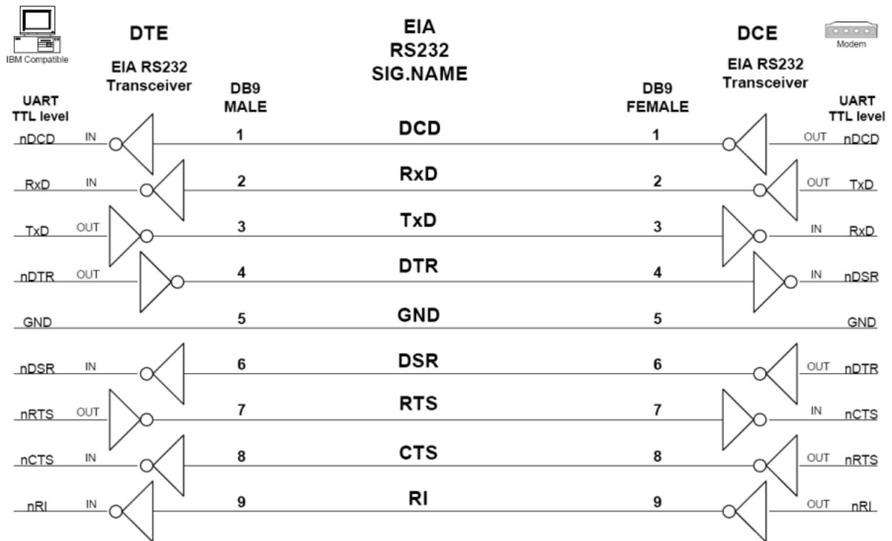
Figure 7: RS232 connections
