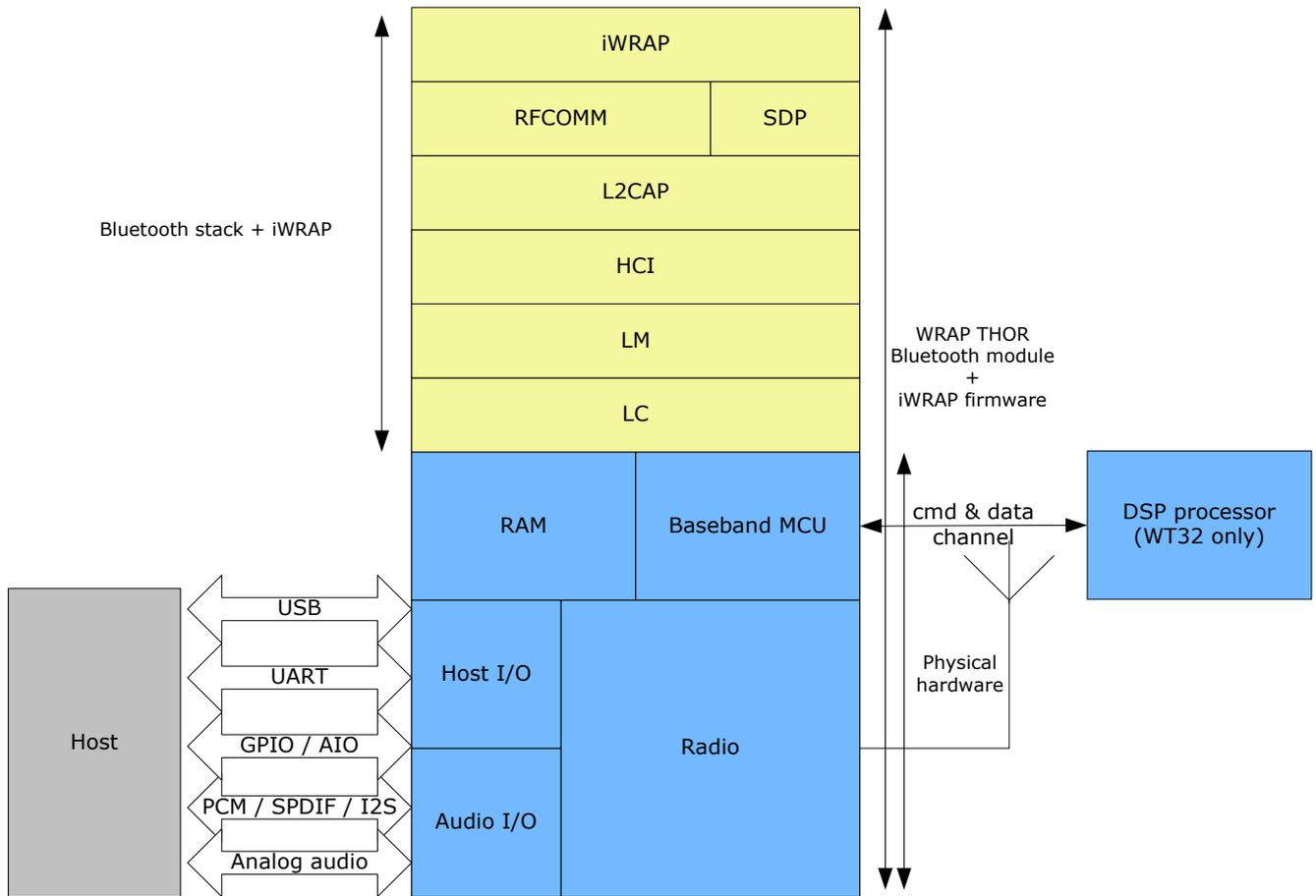
**Figure 1: iWRAP Stack**
