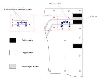
Antenna feed pad indicated. All other pads should be connected to ground.
