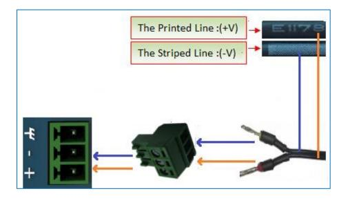
The power supply range is 9 to 26 VDC.
