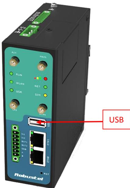
USB interface is used for batch firmware upgrade, cannot used to send or receive data from slave devices which with USB interface.
