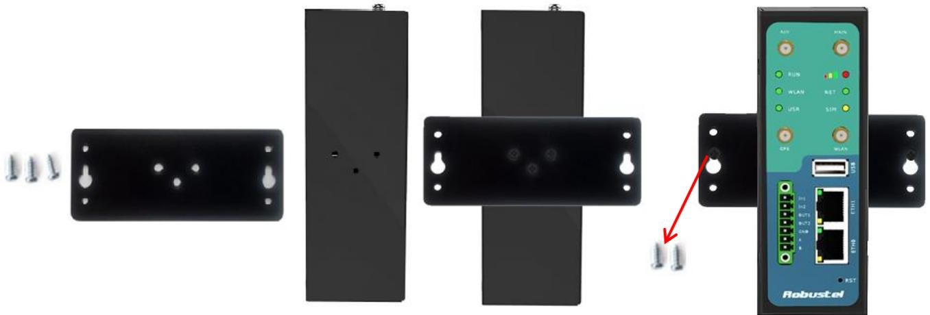
2. Mount the router on a DIN rail with 3 pcs of M3 screws, and then hang the DIN-Rail on the holder.
