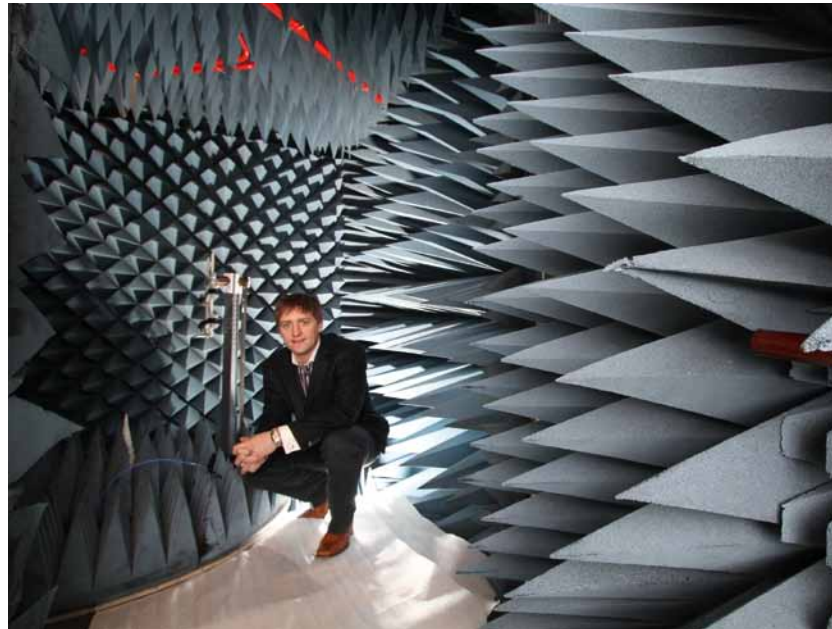
Dermot O'Shea in Taoglas 12M 400-6000MHz ETS Lindgren 3D Tapered Anechoic Chamber
